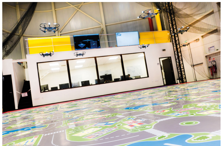
▼ FIG. 1: Test of the bio-inspired flocking model using a swarm of Tello EDU drones in the indoor drone flight arena of the French National School of Civil Aviation in Toulouse, France (David Villa, Sciencelimage, CBI, CNRS, Toulouse).
