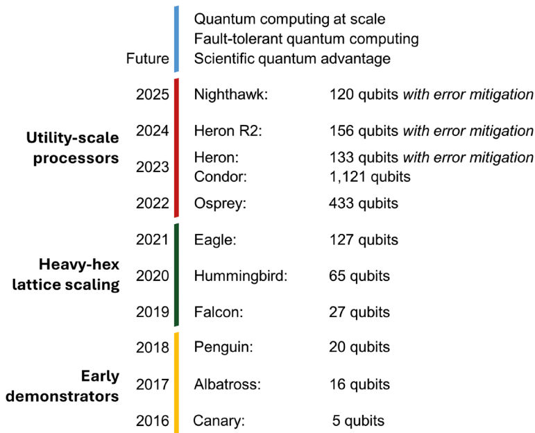
▲ FIG 2: Timeline of major IBM Quantum processor generations over the past decade, showing the progression from early few-qubit demonstrators to utility-scale systems with over a thousand qubits.
