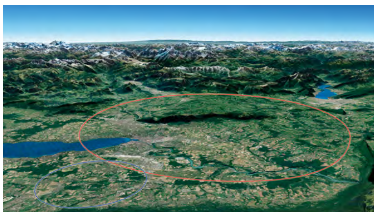
▼ FIG. 2: A schematic view of the possible implementation of the nearly 100 km FCC tunnel. © CERN
