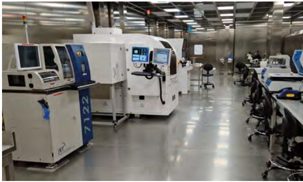
▲ FIG. 2: A detail of the SiPM packaging facility in NOA equipped with a flip chip bonder, a wire bonder, a dicer, and a cryoprobe, which can be operated at 77 Kelvin.
