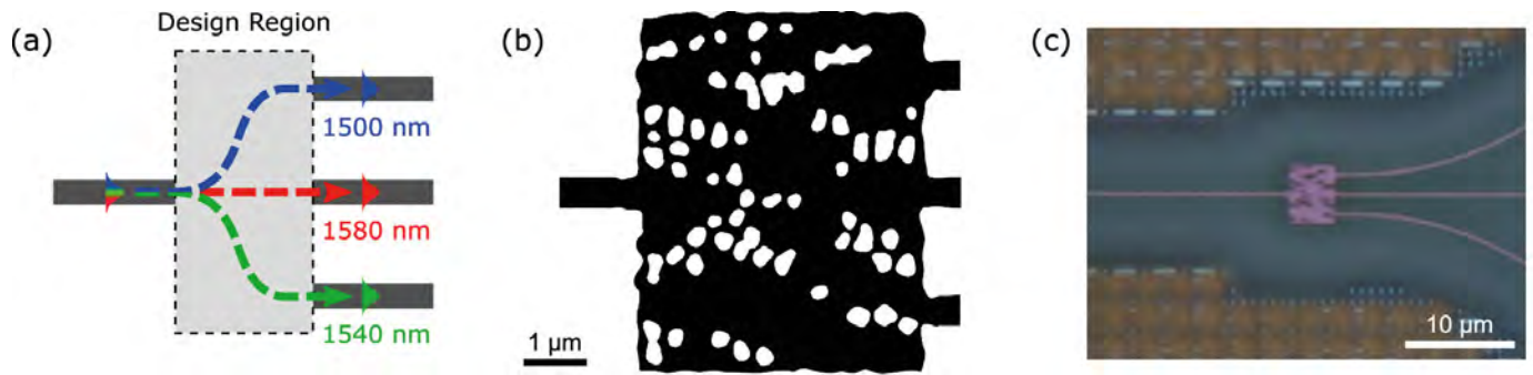
▲ FIG. 2: Manipulation of light. This example illustrates the numerical design of a microscale optical system separating different spectral waves and funnelling them into different waveguides. Adapted from [1] with permission from APS.
