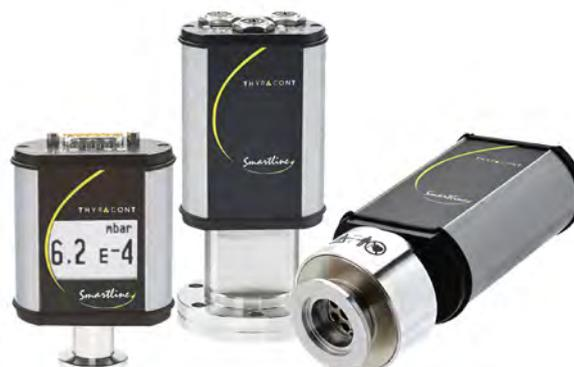
Thyracont's digital Smartline™ transducers with modern combination sensors measure in range of rough to high vacuum, offering outstanding reliability and precision. Beside the classic analogue 0-10V output, their digital interfaces RS485, EtherCAT and Profinet allow intelligent connection to PLCs. Complying with OPC UA, the products grant a safe data transmission from machine to machine or machine to PC, independent of manufacturer, programming language or operating system.
