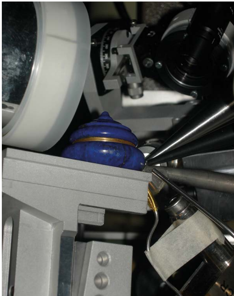
▲ FIG 4: An artwork from the 'Collezione Medicea' during IBA analysis carried out at the external microbeam at INFN-LABEC in Florence.
