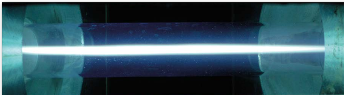
► FIG. 2: CO 2 plasma discharge at 3 kW absorbed power at 500 mbar pressure and 75 standard ltr/min gas flow rate
