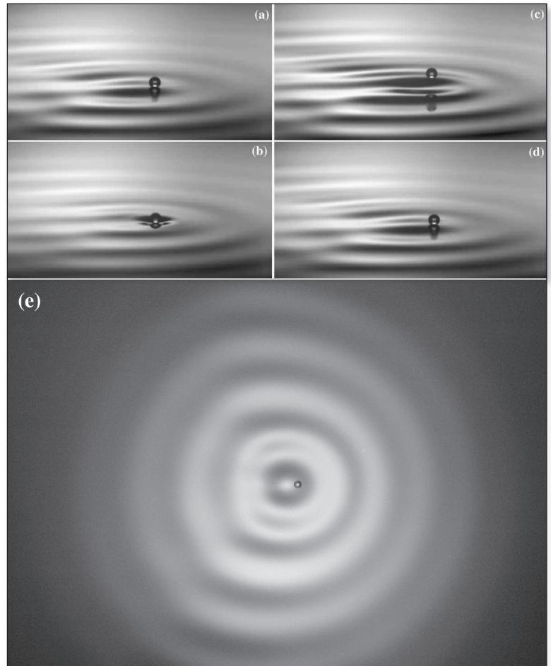
**▲ FIG. 1:** (a-d) Four successive pictures of a walker, side view; (e) top view. Photographs a and d were taken when the droplet touches the surface on the slope of the central bump of the wave generated by the previous collisions. The droplet diameter is approximately 0.7 mm.
