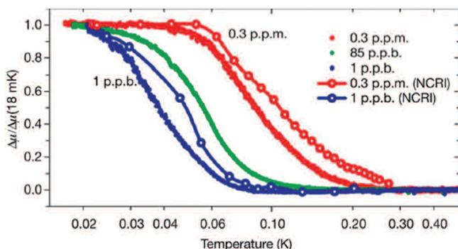
▲ FIG. 3: Shear modulus  $\mu$  of solid  $^4\text{He}$  has an anomalous increase of about 11% going from 300mK to 18mK. The variation  $\Delta\mu = \mu(T) - \mu(300\text{mK})$  normalized to the 18mK value is plotted as a function of  $T$  for samples with different concentration of  $^3\text{He}$  impurities (filled symbols). Open symbols represent similarly scaled NCRI  $\rho_s$  data from torsional oscillator measurements. (Figure from ref. 5)
