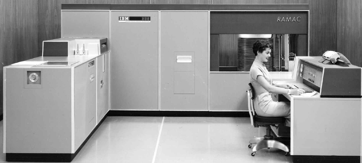
▲ FIG. 1: The IBM 305 RAMAC data processing computer, introduced in 1956, featured the world's first disk storage unit (IBM 350). Photo courtesy IBM.
