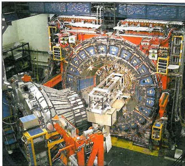
▲ Fig. 4: A photograph of the CDF detector, opened during the installation of the silicon detector. From the inside to the outside, the tracking chamber, the calorimeter and the muon chambers can be seen.
