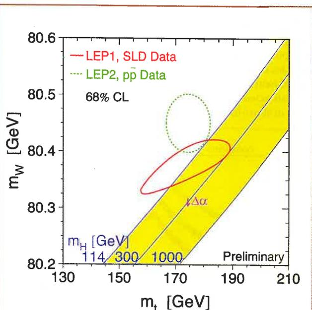
▲ Fig. 2: Masses of the W boson and of the top quark as measured directly at LEP and at the Tevatron (in green), and as indirectly predicted, based on precision measurements at the Z resonance (in red); the contours drawn correspond to a confidence level of 68%. The yellow band represents the Standard Model prediction for various Higgs boson masses. Direct and indirect measurements are in agreement, and point toward a light Higgs boson. (From Ref. 5.)
