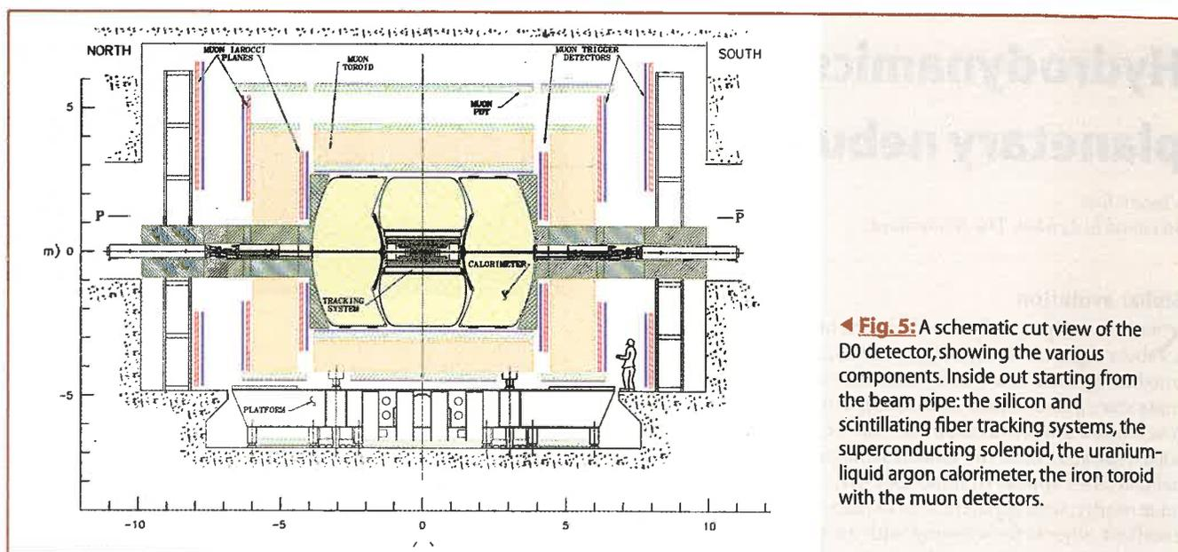
◀ **Fig. 5:** A schematic cut view of the D0 detector, showing the various components. Inside out starting from the beam pipe: the silicon and scintillating fiber tracking systems, the superconducting solenoid, the uranium-liquid argon calorimeter, the iron toroid with the muon detectors.
