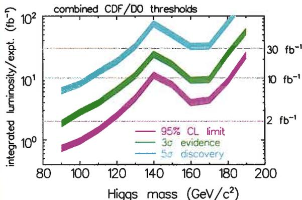
▲ Fig. 3: Reach of the Standard Model Higgs boson search at the Tevatron. The curves represent, as a function of the Higgs boson mass, the luminosity which has to be delivered to each of the two experiments in order to allow an exclusion at 95% confidence level (in purple), a  $3\sigma$  evidence (in green), or a  $5\sigma$  observation (in blue) to be achieved. (From Ref. 7.)
