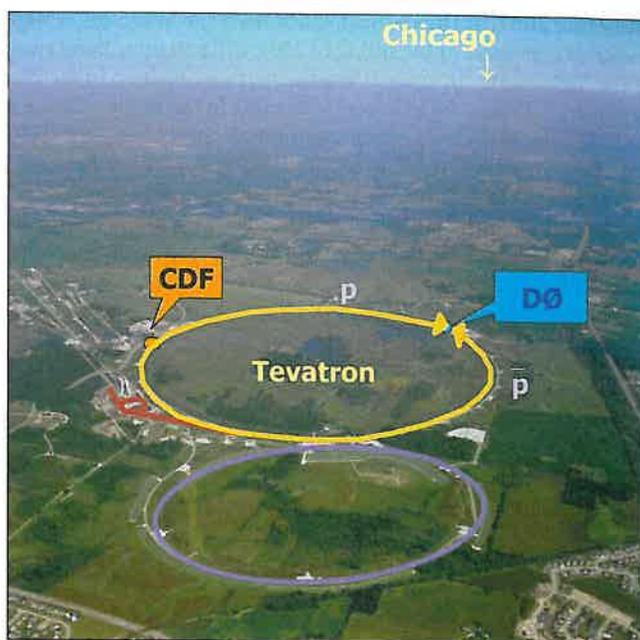
▲ Fig. 1: An aerial view of the Fermilab site. The main components of the accelerator system are highlighted: in yellow, the Tevatron, a 2 TeV proton-antiproton collider; in red the initial injection system; in blue the newly constructed main injector and recycler. The locations of the CDF and D0 detectors are also indicated.
