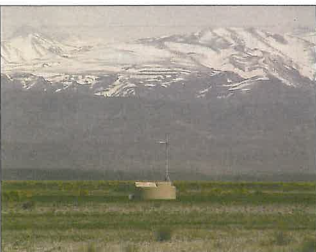
▲ Fig. 4: One of the detector stations of the Auger Observatory in the Argentine Pampa (the Andes in the background). The complete ground array will have 1600 such stations spread over a surface of 3000 km 2 . A typical cosmic ray induced airshower in the relevant energy range covers an area of several tens of km 2 with some 100 billions of secondary particles (mainly photons and electrons) that reach the ground level. The detector stations (tanks filled with 12 tons of pure water where the charged particles produce Cherenkov light) sample the shower particles, count their number and put a time tag on them. It is then possible to reconstruct the energy and direction of the primary cosmic ray. Each station is autonomous, powered by solar panels, and communicating with a central computer more or less through cellular-phone-like techniques.
