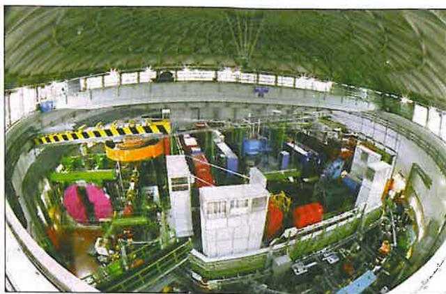
▲ **Fig. 5:** A fish eye view of the DAΦNE hall at LNF (Frascati National Laboratory). The DAΦNE accelerator has a circumference of about 190 m and two interaction regions: IP1, on the right side of the picture, is presently occupied by the KLOE experiment devoted to CP violation studies; IP2, on the left, is the FINUDA interaction region. The FINUDA detector, the assembly with dark pink octagonal end-caps, will be moved onto the beam line next autumn.
