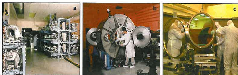
◀ Fig. 2: The VULCAN laser facility at the RAL near Oxford, UK. a) Part of the VULCAN laser Nd:glass amplifier chain. b) The interaction chamber used for nuclear experiments. c) Installation of the optics for the new Petawatt upgrade.
