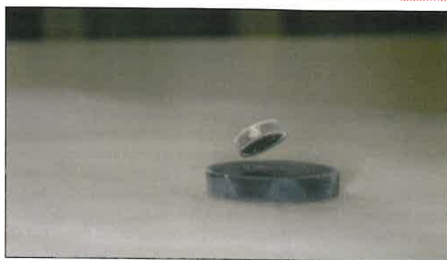
Fig. 3: Superconductors exclude magnetic flux (the Meissner effect). A magnet lowered towards a superconductor will 'see' an identical magnet the same distance below the surface due to supercurrents induced on the superconductor surface. The resultant repulsive force levitates the magnet, provided that the force is greater than the magnet's weight. Magnetic levitation (Maglev) trains and frictionless superconductor bearings use this repulsive force. Here a neodymium-iron-boron magnet floats above a disk of lead-doped BSCCO superconductor, with a critical temperature T_c of 108 K. The superconductor has been cooled in liquid nitrogen, and the magnet falls when the superconductor is warmed above T_c .
