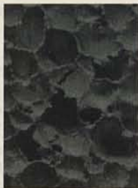
The cover image is a ten-times magnification of a metal foam see page 17
