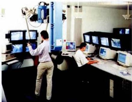
The picture on the cover of this special issue was taken inside the activated environment of the JET fusion tokamak in the UK. It shows the end of a robotic arm recently used to insert an improved divertor (the 'exhaust') in the floor of the tokamak, following the 1997 experiments described in chapter 4.4. The arm was handled remotely (above)—the first use of remote handling in a fusion reactor.
