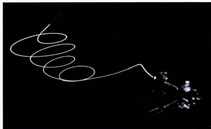
Photograph of the 1.1 Watt continuous wave up-conversion fibre laser showing the pump input coupling optics, the fibre, and the red output (dark grey fibre tip, top left of picture)
