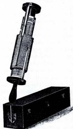
Fig 3 The spiral slide rule designed by George Fuller, mounted on its carrying box for convenience. Made by W.F. Stanley of London from the late 19th century until well into this century. It is equivalent to a straight slide rule over 25 metres long
