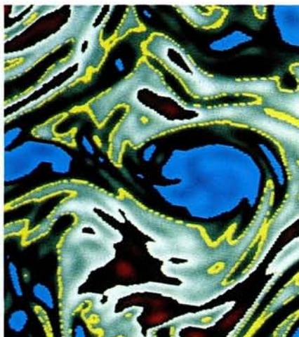
Left: The complex multiple scale structure of very turbulent flow is revealed by passing a two-dimensional sheet of laser light across a jet seeded with fluorescent dye (Sreenivasan and Prasad, 1989). Right: A computer-generated image of a numerical simulation of turbulent flow showing a multi-fractal structure (Farge and Sadoury, 1989). It bears a striking resemblance to the observed structure, which is fractal and independent of the large flow pattern at an intermediate range of sizes.
