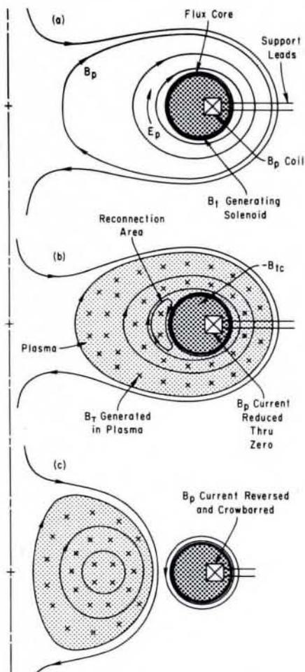
Fig. 4 — The S-1 inductive formation method begins with (a) the plasma linked to the flux core. As currents are induced into the plasma (b) reconnection occurs and (c) the spheromak separates from the structure.
