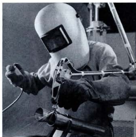
Fig. 1 — 400 W flexible laser beam guide (12mm bore).
