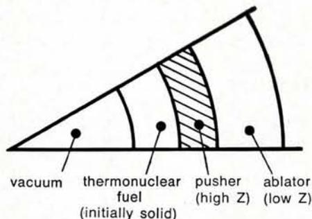
An improvement proposed by people from the Lebedev Institute in Moscow is a thin layer of high Z material inserted inside the thermonuclear fuel to stop any unwanted suprathermal electrons created in the corona.
