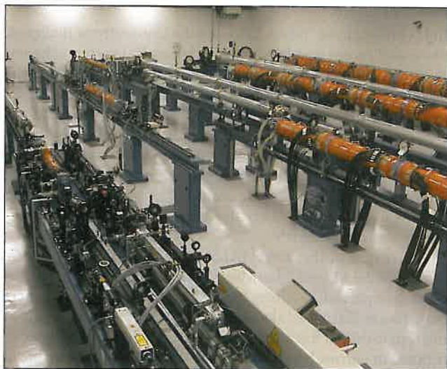
▲ Photo: View of the chain of PALS laser amplifiers, with an oscillator block in the foreground.
