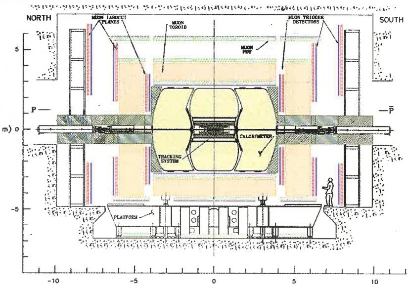
**Fig. 5:** A schematic cut view of the D0 detector, showing the various components. Inside out starting from the beam pipe: the silicon and scintillating fiber tracking systems, the superconducting solenoid, the uranium-liquid argon calorimeter, the iron toroid with the muon detectors.
