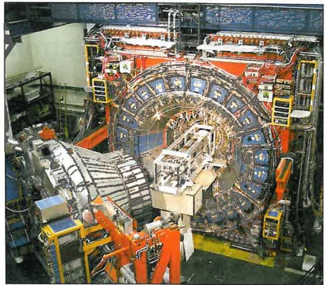
**▲ Fig. 4:** A photograph of the CDF detector, opened during the installation of the silicon detector. From the inside to the outside, the tracking chamber, the calorimeter and the muon chambers can be seen.
